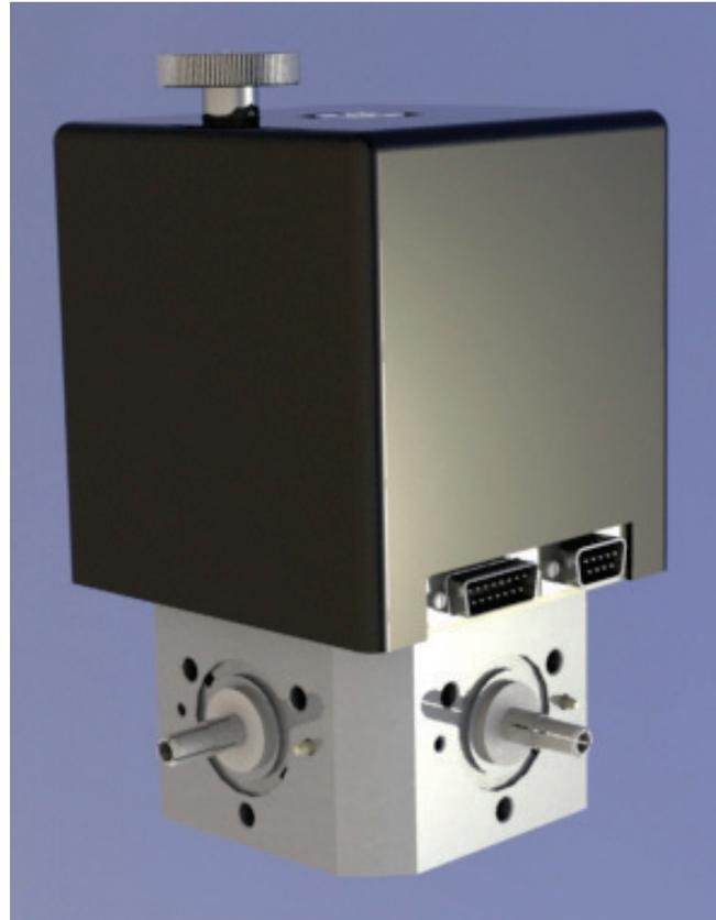
The models SW78.01, SW 78.02 and SW 78.03 are motor-driven, two-way coaxial transfer switches designed to change coaxial connections with a minimum off-air-time. Mainly they are used for switching transmitters, antennas, dummy loads and other peripheral equipment in situations when broadcasting procedures are modified, when there is need for emergency repair, or during scheduled maintenance.
